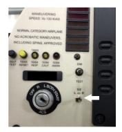
Well, now YOU CAN have your cake and eat it too! Jim has developed a precision Dual TIT Probe Indication Kit that allows you to simply flip a switch to get a readout for either left or right TIT probes!
